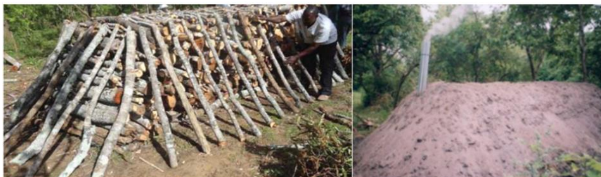
Figure 14: Charcoal production - improved earth mound kiln in Kilosa
