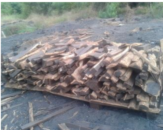
Figure 1. A pile of wood off-cuts from Dalbergia melanoxylon arranged to be covered with earth to form an earth mound charcoal kiln (Source: URT, 2019).
