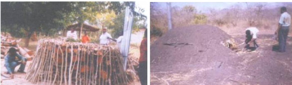
Figure 5. Improved Earth Mound Kiln at Ruvu Fuellwood Pilot Project, Coast Region, Tanzania.
