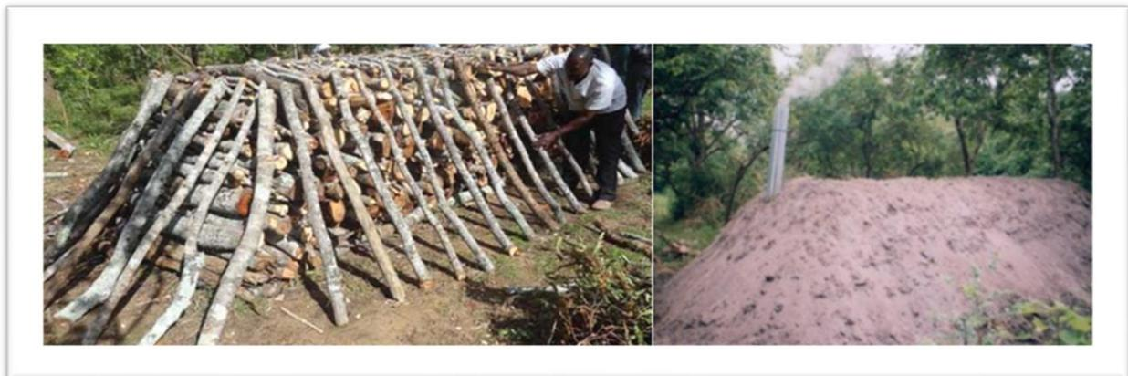
Figure 19: Improved earth mound kiln (IEMK) for charcoal production in Kilosa<sup>54</sup>
